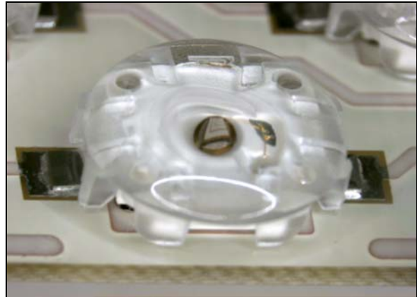
Figure 13: Good solder connection / laser soldering
